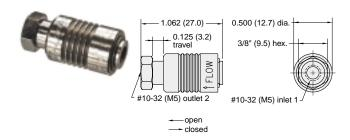
Medium: Air, Water or Oil Mounting: Inline or direct to fitting
